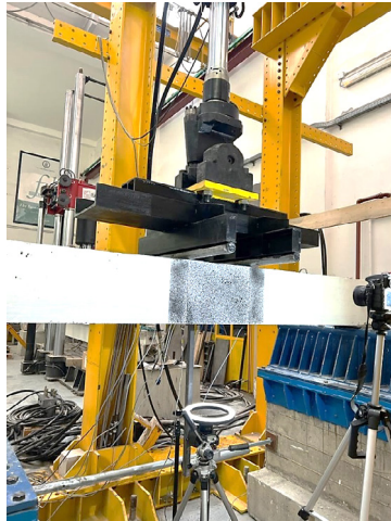
FIG. 20.3 - FATIGUE TEST SET UP
