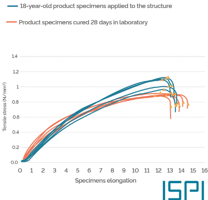
FIG. 20.7 - COMPARISON OF TENSILE STRESS AND ELONGATION VALUE BETWEEN MATERIAL SPECIMENS CURED 28 DAYS IN LABORATORY AND THOSE AGED 18 YEARS
