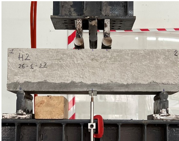
FIG. 20.1 - RESTORED SPECIMENS UNDER FLEXURAL TEST
